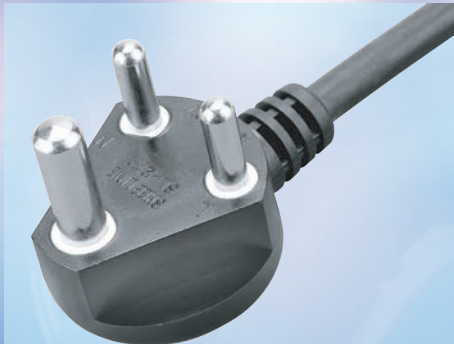
SL-27A (For Use In India) H03VVH2-F, H05VVH2-F 0.75mm 2 /2C H03VV-F, H05VV-F 0.75mm 2 /3G H05VV-F 1.0~1.5mm 2 /3G H05RN-F 0.75~1.0mm 2 /3G
