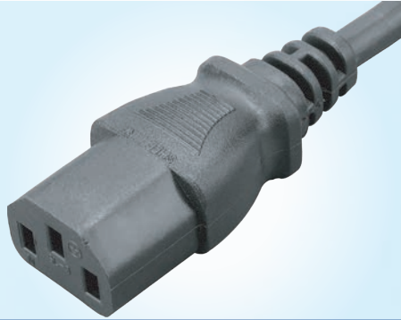
SL-3 (IEC 320 C13) SJT 18~14AWG/3C SVT 18AWG/3C H05VV-F 0.75~1.5mm 2 /3G
