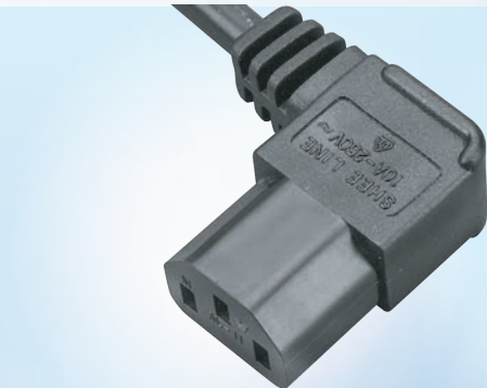
SL-11 (IEC 320 C13) SJT 18~14AWG/3C SVT 18AWG/3C H05VV-F 0.75~1.5mm 2 /3G
