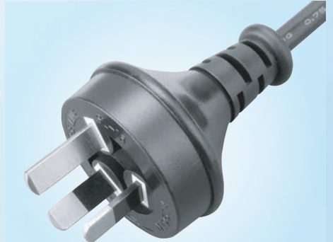
SL-16 (SAA)Australia Plug(AS/NZS 3112) H03VV-F 0.75mm 2 /3G H05VV-F 0.75~1.5mm 2 /3G H05VVRN-F 0.75~1.0mm 2 /3G
