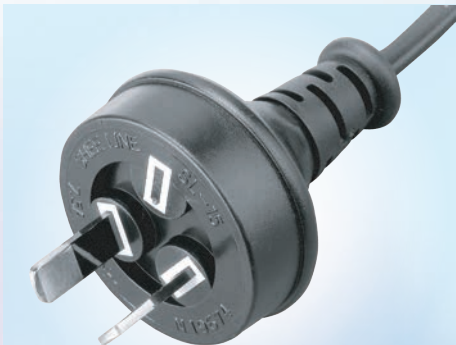
SL-15 (SAA)Australia Plug(AS/NZS 3112) H03VVH2-F 0.75mm 2 /2C H05VVH2-F 0.75mm 2 /2C H05VV-F 0.75~1.0mm 2 /2C
