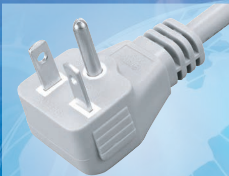
SL-202 (NEMA 6-20P) VCT3.5mm 2 /3C VCTF 1.25~2.0mm 2 /3C
